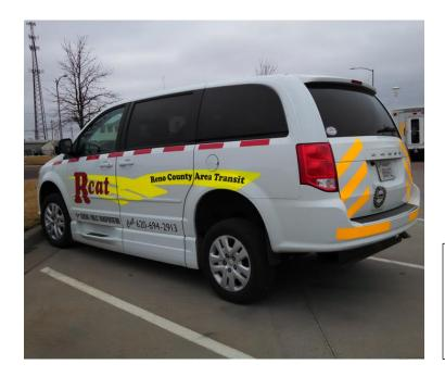
For safety, all Rcat vehicles graphics are made from highway grade reflective film and tape. Red and white conspicuity tape is applied nose to tail along with safety yellow florescent chevrons on the back.
